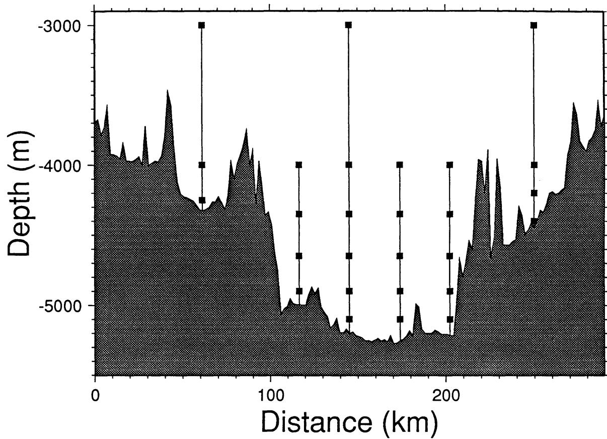
**Figure 3.** The mooring array in the Samoan Passage and underway bathymetry. The perspective is looking northward, so mooring 1 is on the left and mooring 6 is on the right. The squares indicate the locations of current meters.
