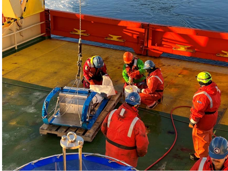
Figure 11. Successful sled deployment, note the clean nets and the codend going into the bucket. Photo by Heather Jackson.
