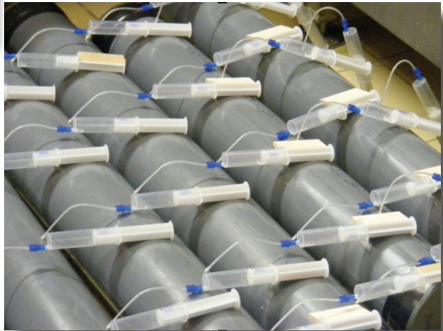
Fig. 8.8: Pore water sampling of GC segments
