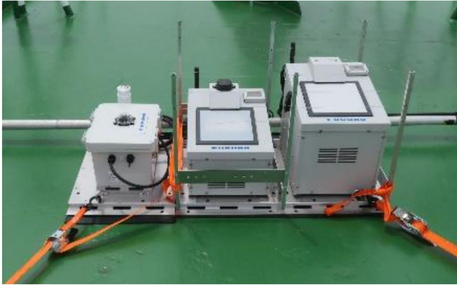
Fig. 3.9-1: Outlook of the instruments installed at the roof of the aft wheelhouse; the microwave radiometer for the air temperature (right), microwave radiometer for the water vapor (middle), and the whole-sky camera (left).
