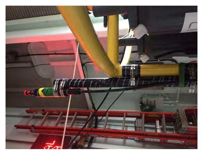
Fig. 1: Upward-looking chipod sensor attached to the rosette
