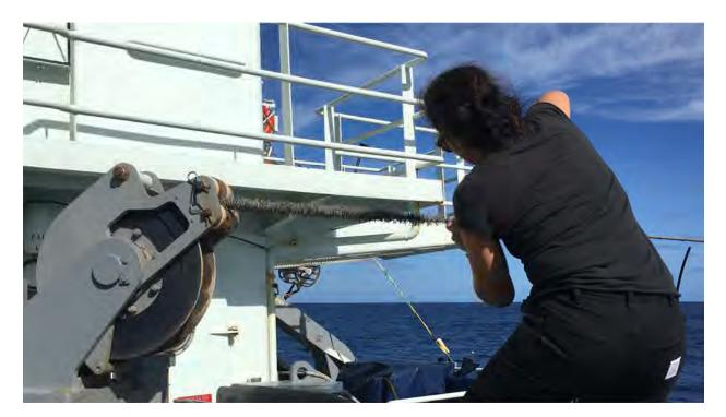
Fig. 6: Birdcage of approximately 100 meters of wire forming outside of the level wind intake being freed by RV Thompson marine technician Jen Nomura.
