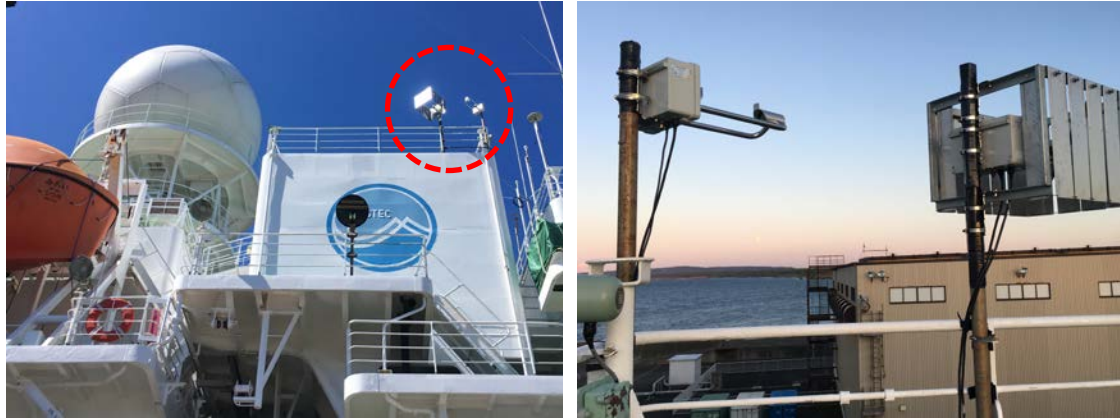
Fig. 3.7.1-1: Onboard LPM sensors. (Left) The location of the sensors, as designated by the red broken circle. (Right) The sensors. Right one (aft one) equipped wind protection element to reduce the effect of the wind, while left one (fore one) did not.
