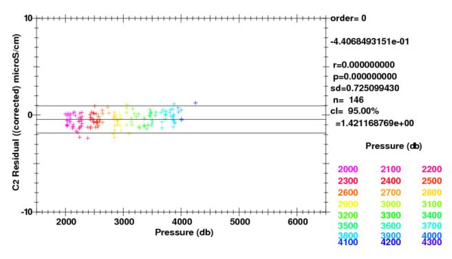
Fig. 3.43: Deep Corrected  $C_{Bottle}$  - C2 by pressure (Pressure >= 2000dbar).
