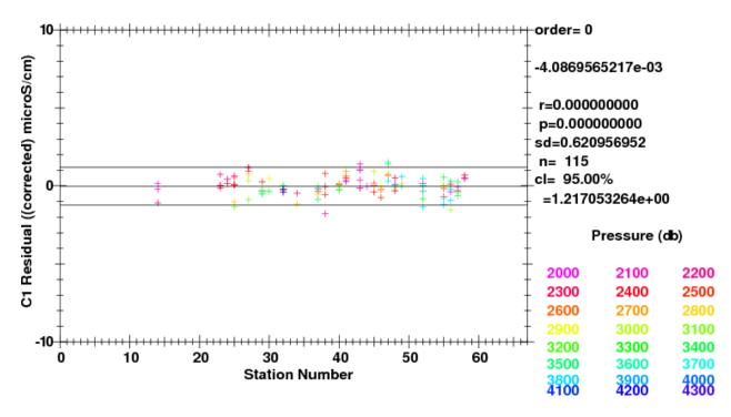
Fig. 3.37: Deep Corrected  $C_{Bottle}$  - C2 by station (Pressure >= 2000dbar).
