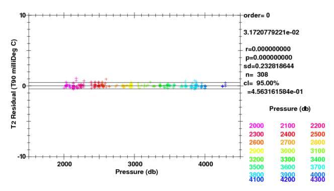
Fig. 3.19: SBE35RT-T2 by pressure (Pressure  $\geq$  2000dbar).
