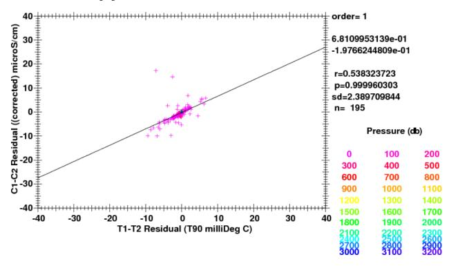
Fig. 3.22: Coherence of conductivity differences as a function of temperature differences.
