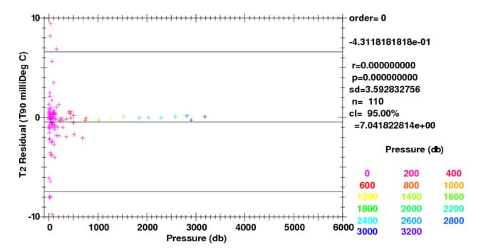
Fig. 3.6: SBE35RT-T2 by pressure  $(-0.002^{\circ}\text{C} \le \text{T1-T2} \le 0.002^{\circ}\text{C})$ .
