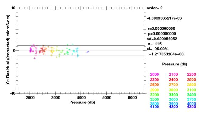
Fig. 3.41: Deep Corrected  $C_{Bottle}$  - C1 by pressure (Pressure >= 2000dbar).
