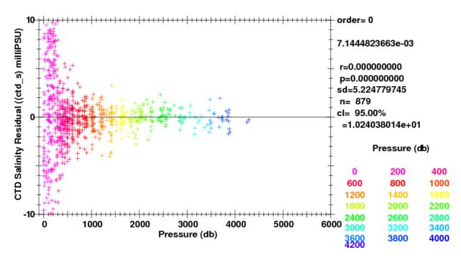
Fig. 3.46: Salinity residuals by pressure  $(-0.002^{\circ}\text{C} \le \text{T1-T2} \le 0.002^{\circ}\text{C})$
