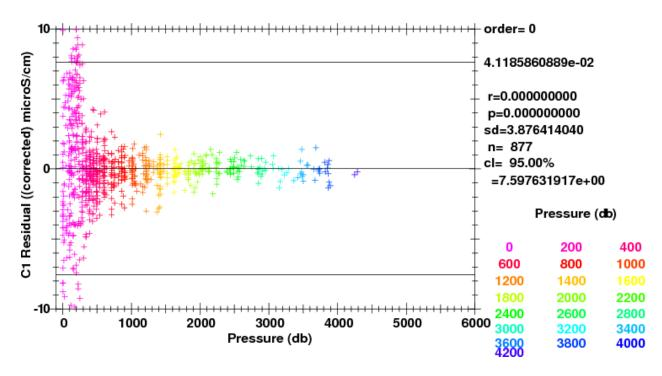
Fig. 3.40: Corrected  $C_{Bottle}$  - C1 by pressure (-0.002°C  $\leq$  T1-T2  $\leq$  0.002°C).
