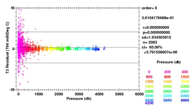
Fig. 3.18: SBE35RT-T2 by pressure  $(-0.002^{\circ}\text{C} \le \text{T1-T2} \le 0.002^{\circ}\text{C})$ .
