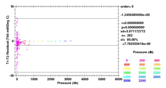
Fig. 3.8: T1-T2 by pressure  $(-0.002^{\circ}\text{C} \le \text{T1-T2} \le 0.002^{\circ}\text{C})$ .
