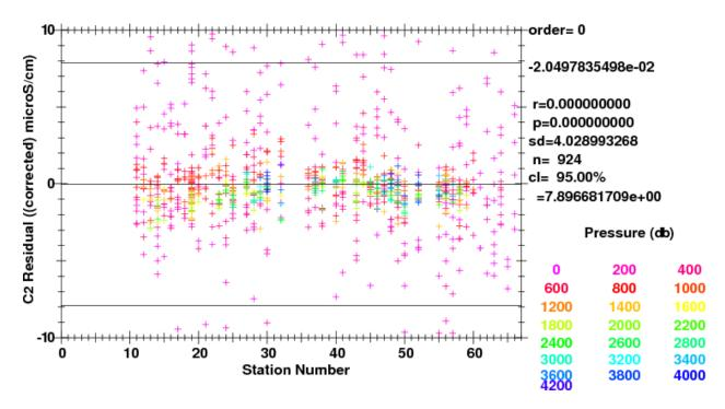
Fig. 3.38: Corrected  $C_{Bottle}$  - C2 by station (-0.002°C  $\leq$  T1-T2  $\leq$  0.002°C).
