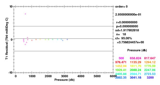
Fig. 3.5: Deep SBE35RT-T1 by station (Pressure  $\geq$  500dbar).
