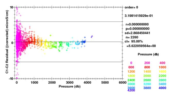
Fig. 3.44: Corrected C1-C2 by pressure  $(-0.002^{\circ}\text{C} \le \text{T1-T2} \le 0.002^{\circ}\text{C})$ .
