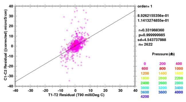
Fig. 3.35: Coherence of conductivity differences as a function of temperature differences.
