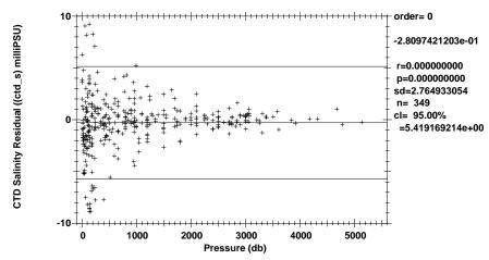
**Figure 1.6.3.17** Salinity residuals by pressure (-0.01°C ≤T1-T2≤0.01°C).
