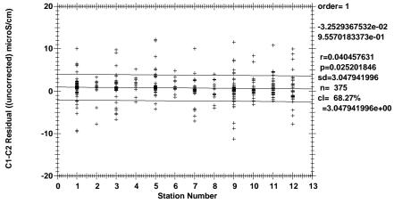
**Figure 1.6.3.1** SIOR Uncorrected C1 - C2 by station (-0.01°C  $\leq T1 - T2 \leq 0.01$ °C).
