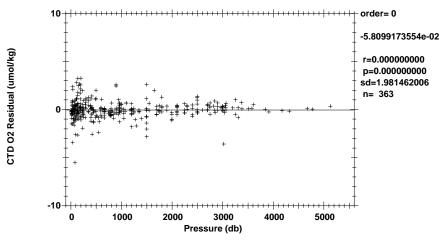
**Figure 1.6.4.1**  $O_2$  residuals by pressure (-0.01°C  $\leq$ T1-T2 $\leq$ 0.01°C).
