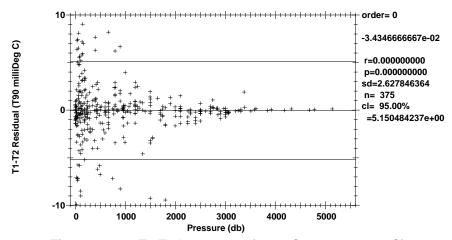
**Figure 1.6.2.3** T1-T2 by pressure  $(-0.01^{\circ}\text{C} \le T1 - T2 \le 0.01^{\circ}\text{C})$ .
