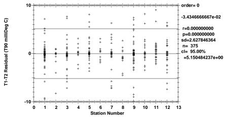
**Figure 1.6.2.0** T1-T2 by station (-0.01°C  $\leq T1 - T2 \leq 0.01$ °C).
