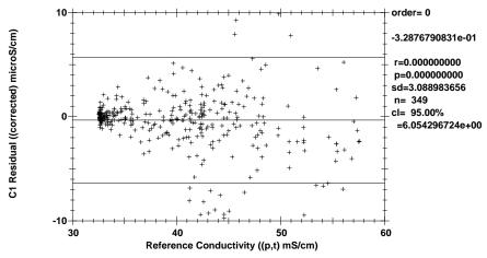
**Figure 1.6.3.14** SIOR Corrected  $C_{\textit{Bottle}}$  – C1 by conductivity (-0.01°C  $\leq$ T1-T2 $\leq$ 0.01°C).
