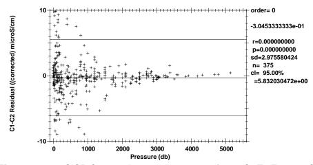
Figure 1.6.3.10 SIOR Corrected C1 - C2 by pressure (-0.01°C  $\leq$ T1-T2 $\leq$ 0.01°C).
