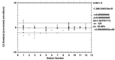
**Figure 1.6.3.9** SIOR Deep Corrected  $C_{Bottle}$  – C2 by station (Pressure >= 1000dbar).
