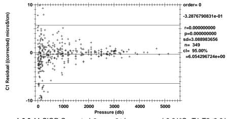
**Figure 1.6.3.11** SIOR Corrected  $C_{Bottle}$  – C1 by pressure (-0.01°C  $\leq$ T1-T2 $\leq$ 0.01°C).
