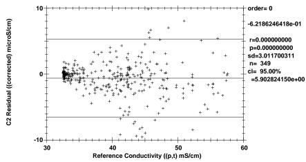
**Figure 1.6.3.15** SIOR Corrected  $C_{Bottle}$  – C2 by conductivity (-0.01°C  $\leq$ T1-T2 $\leq$ 0.01°C).
