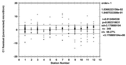
**Figure 1.6.3.2** SIOR Uncorrected  $C_{Bottle}$  – C1 by station (-0.01°C  $\leq T1 - T2 \leq 0.01$ °C).
