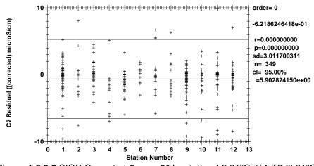
**Figure 1.6.3.8** SIOR Corrected  $C_{Bottle}$  – C2 by station (-0.01°C  $\leq$ T1-T2 $\leq$ 0.01°C).
