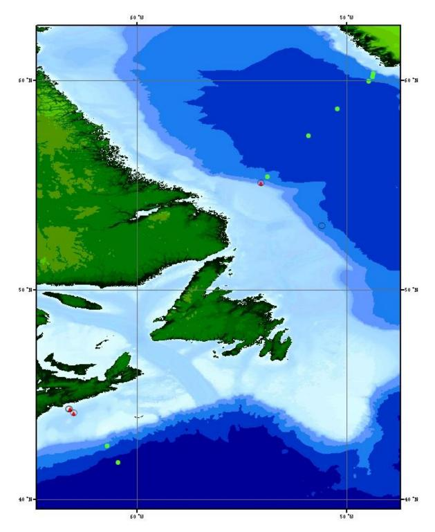
Figure A.2.3 Mooring operations (red-filled triangles are moorings deployed; black hollow circles are moorings recovered) and float deployment locations (green-filled circles) for HUD2008009.
